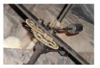
9. \_\_\_\_\_: the gears to drive and balance the hands require regular maintenance.
