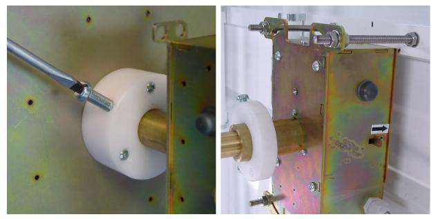
The T300 may be centre fixed using an adjuster boss and mounting plate, or frame fixed via the four mounting holes on the chassis. This makes the T300 adaptable for solid or backlit dials.
