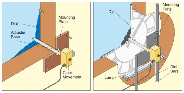
T300 installed on a mounting plate with adjuster boss to accommodate wall thickness or backlighting.
