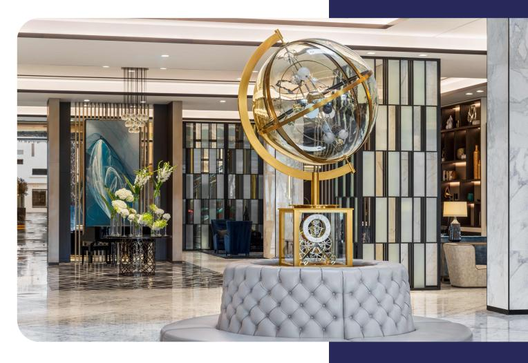
Situated in the lobby of the newly opened Waldorf Astoria Kuwait, which opened its doors on the 24th August 2022, the clock features a sphere made from eight pieces of compound curved glass panels and brush polished stainless steel parts with a gold PVD finish. Drawing on the conceptual design initiated by LW Design our Smith of Derby design team worked closely with LW to refine the design and create an iconic time-piece in a contemporary style, which reflects the traditional Waldorf clock.
