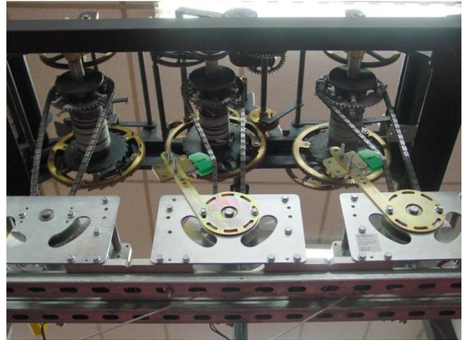
The AW10 units are installed on a separate frame which can be located above or below the clock mechanism. The split barrel sprockets have a special method of clamping to the clock barrel.
