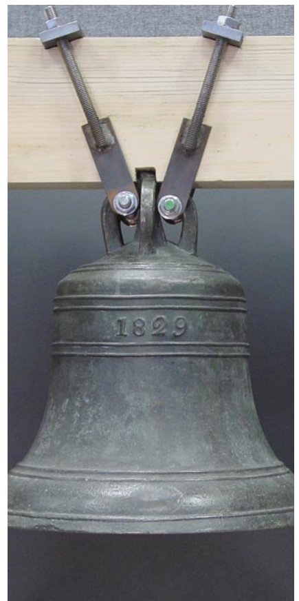
Example of a bell with crown and fixing rods.
