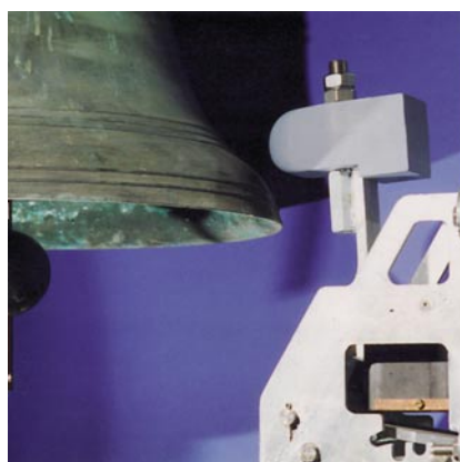
External electro-magnetic hammer in-situ.
