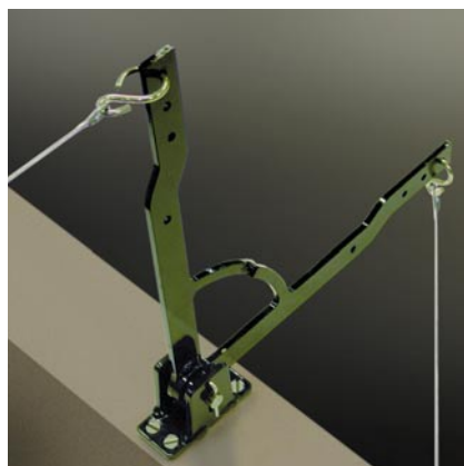
Right-angle lever for hammer connecting wire.
