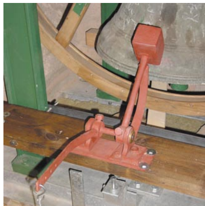
Typical hammer assembly unit.
