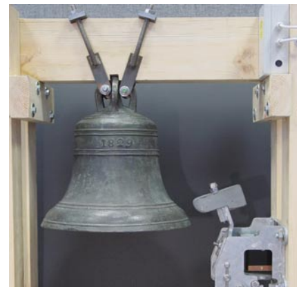
Re-hung bell, replacement hangers & EMH.
