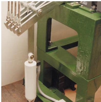
Electrical Actuator Pull-Off (APO series).
