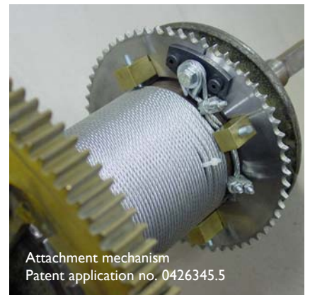
A clock main barrel with AW8 sprocket fitted. Note the securing clamps and pads which require no holes to be drilled in the original barrel. The cable is tensioned to stabilise the sprocket and prevent slippage.
