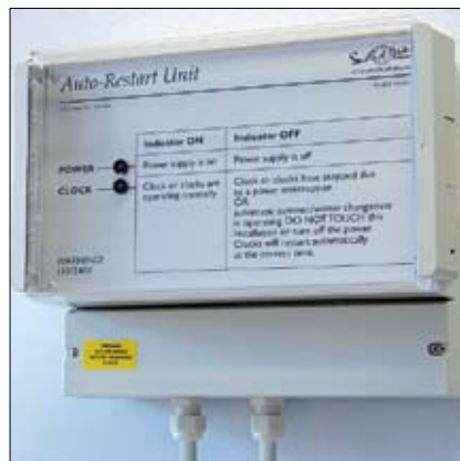
Auto-Restart back-up option for synchronous clock movements.
