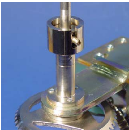
Ball and socket type expansion joint on a vertical transmission rod.
